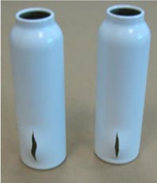
Monobloc can tested by Buckle & Burst (bursts at 30 PSI)
