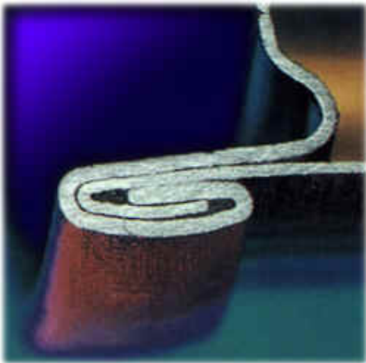
The seam - close up.
