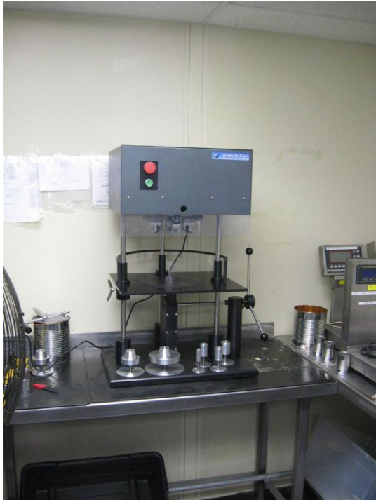
The Seam Stripper at a large cannery
