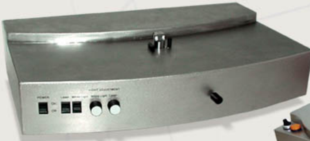
Laser light profiles the outside of the capsule for measuring the diameter at two points.
