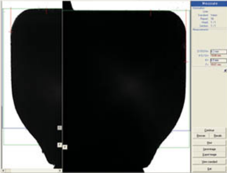
Laser light profiles the outside of the capsule for measuring the diameter at two points.
